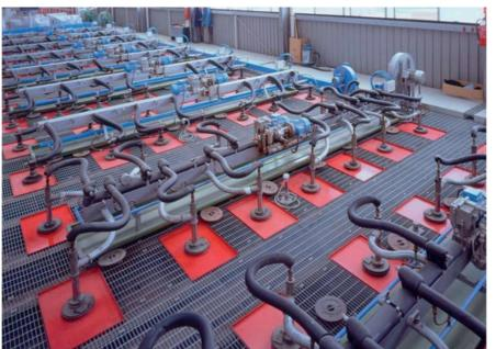
The NIR/4 burner works with atomized fuel impulses and every group can feed a maximum number of 16 fi ring points; the impulses frequency and power is managed by an inverter controlled motor. All feeders are equipped with fuel heater. The NIR/4 burners can be supplied complete with switchboard and, on demand, they can be completed by a blowing manifold for the nozzles cooling, in case they would be used on kilns working in pressure.
