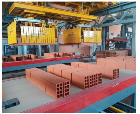
Experience and deep knowledge of the production cycle allows us to design unloading fired product systems that have high precision, rapidity and synchronism. They can be both robotized or orthogonal and of high versatility in order to manage any type of product.
