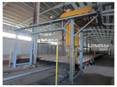
COSMETEC AUTOMATION plans and realizes kiln cars handling systems and cars automatic cleaning and greasing systems.
