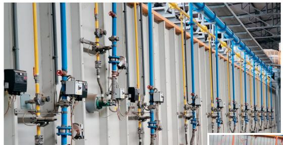
THE BLG/1 BURNER can be supplied with combustion air fan for each firing point.
